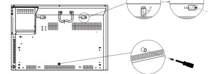
1.Insert the bracket(to the hole),turn it anticlockwise 90°, fasten it with screw; 2.Press the rubber pad (in the hole), fasten it with screw.
