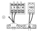
b) Wire routing of unified power supply:
