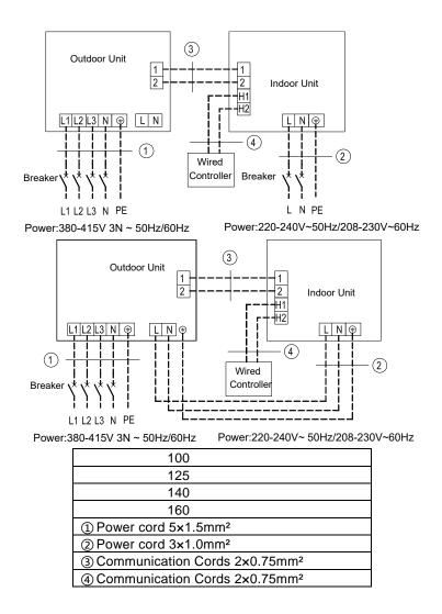
(5) Electrical wiring of indoor unit and Electrical wiring of outdoor unit
