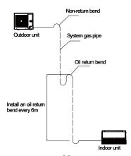
Dimensions for the making of oil return bend are as follows:
