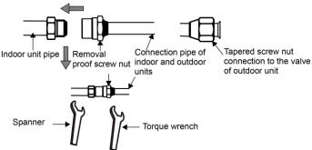
Installation method: Connect the connection pipes first to the indoor unit and then to the outdoor unit. When bending a connection pipe, be careful not to damage the pipe. Do not over-tighten the screw nut, otherwise leakage will occur. Besides, the outside of connection pipe should be added with a layer of insulating cotton to protect it from mechanical damage during installation, maintenance and transportation.
