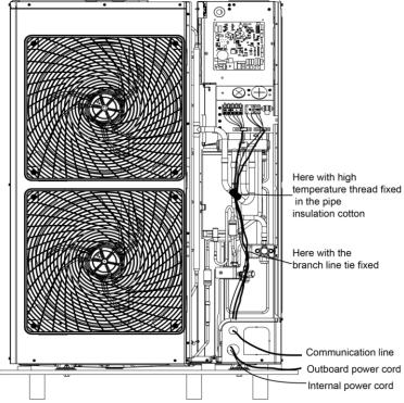
Power cord should be secured along with the right side plate and fixed to the hook with a wire clamp so as to avoid contacting the pipeline. The communication line between indoor and outdoor units should also be laid along with the right side plate but away from the power cord.
