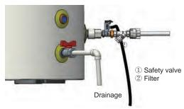
Installation Mode 1 of the Tap Water Safety Valve (Inlet Water Pressure =0.1~0.5MPa)
