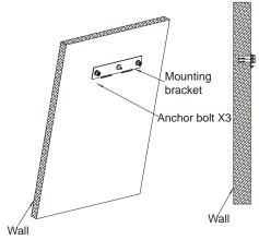
Step3: Attaching indoor unit to the wall.
