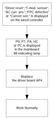
◆ IPM or PFC Over-temperature Protection(Code:"P8")
