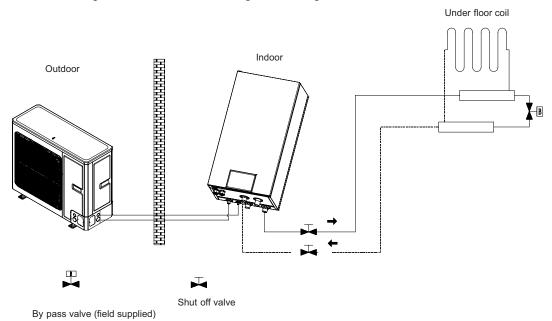
Note: the bypass valve must be installed to secure enough water flow rate, and should be installed at the
