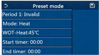
The option "Mode" is used to preset the mode; "WOT-Heat" is used to set the leaving cold/hot water temperature; "Start timer"/"End timer" is used to for time setting. After that, by touching the "Save" icon, all settings will be saved.
