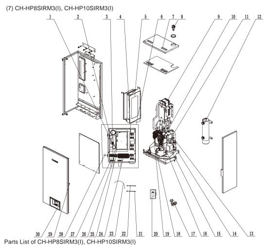
No Name of part Quantity Display Board Magnet Sub-assy Jumper Main Board Mounting board Terminal Board Terminal Board Communication line Temperature Sensor Temperature Sensor Remote room temperature sensor Water Pump Flow switch Strainer Sealing Cap(Pressure Warning) Electric starter of water valve Electric three-way ball valve body Relief Valve Electric Heater Drainage Pipe Sub-assy Water Pressure Gauge
