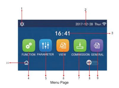
Above the menu, the corresponding icon will be displayed based on the mode and status of the controller.
