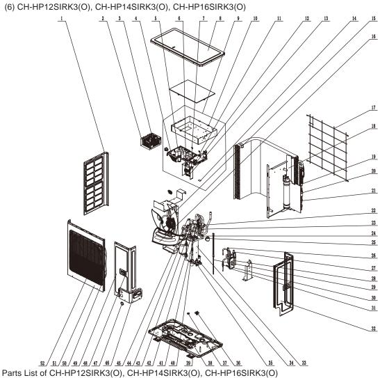
No. Name of part Quantity Left Side Plate Inductance Box Assy Inductance Radiator Drive Board Terminal board Filter Board Coping Electric Box Assy Electric Box Main Board Communication Interface Board Electrical Retaining Plate Jumper Brushless DC Motor Axial Flow Fan Rear Grill Condenser Assy Current Divider Silencer Strainer Pressure Sensor Nozzle for Adding Freon
