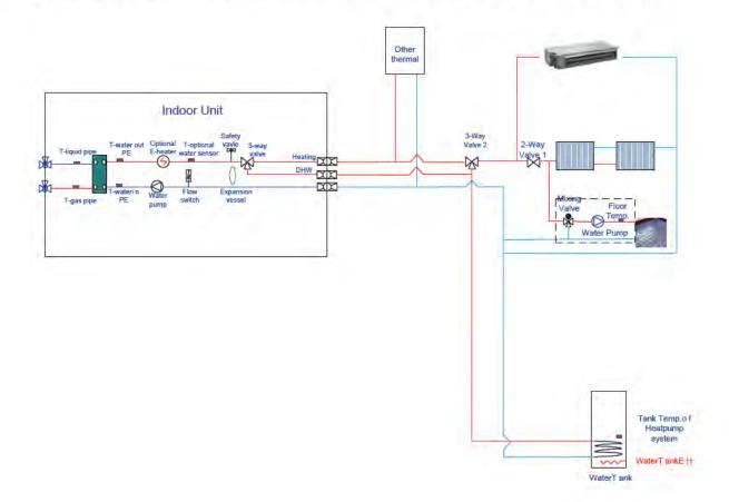
◆ CH-HP12SIRK3,CH-HP14SIRK3,CH-HP16SIRK3,CH-HP8.0SIRM3, CH-HP10SIRM3, CH-HP10SIRM3, CH-HP14SIRM3, CH-HP16SIRM3 (Water tank with the external plate-type heat exchanger)
