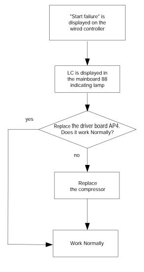
◆ Compressor Current Protection (Code:"P5"); Compressor Motor Desynchronizing (Code:"H7"); IPM Protection (Code:"H5"); Phase Loss (Code:"LD")
