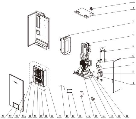
Parts List of CH-HP12SIRK3(I), CH-HP14SIRK3(I), CH-HP16SIRK3(I)
