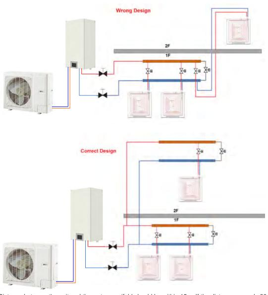
(5) Distance between the unit and the water manifold should be within 15m. If the distance exceeds 20m, then it is required to calculate the hydraulic power.
