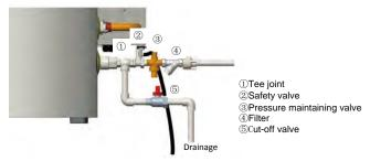
Installation Mode 3 of the Tap Water Safety Valve (Inlet Water Pressure>0.5MPa)
